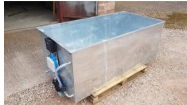
Galvanised steel curing tank c/w digital control, Heating element and circulating pump
